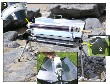
• Find the aiming spike shown in picture (3) and adjust the position of your cooker again until the spike casts no shadow. Your cooker will then be pointing directly at the sun. Make sure the knobs (2) are done up again (firmly but not too tightly) once your cooker is in the correct position. Remember that you will need to aim your cooker at the sun again every 15 to 20 minutes as it travels across the sky. Now turn your cooker away from the sun or shade it until you are ready to cook.
