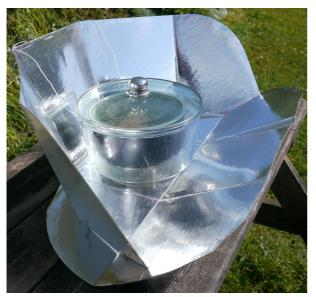
(below, left). Push the two outer wings through the slits and use the two clips provided to adjust the angle of the front flap (below, right). Put your CooKit on a flat horizontal surface, facing the sun. You can use any dark coloured metal cooking vessel with your CooKit, but vessels that are a) matt black in colour and b) as light (i.e. not heavy) as possible work best. You should use a short stand or trivet to keep your cooking vessel off the bottom of your 'greenhouse'. The 'greenhouse' is
